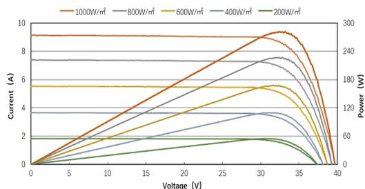
Excellent performance at 200W/m<sup>2</sup>(AM 1.5, 25°C): the conversion efficiency could be 96.6% of STC
