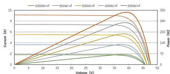
Excellent performance at 200W/m<sup>2</sup>(AM 1.5, 25 °C): the conversion efficiency could be 96.5% of STC
